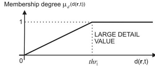
Figure 2: The membership function  $\mu_d$  of the fuzzy set “large detail value”.
