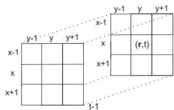
Figure 1: The  $3 \times 3 \times 2$  filtering window consisting of  $3 \times 3$  pixels in the current frame and  $3 \times 3$  pixels in the previous frame.
